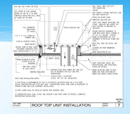
CURRENT DESIGN OF ROOF TOP MECHANICAL UNIT INSTALLATION
